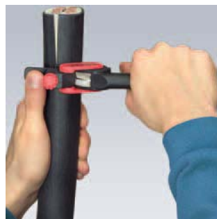
Turning the tool for circumferential cut
