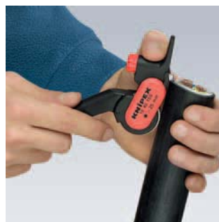
Setting the tool for longitudinal cut
