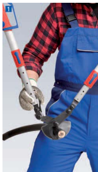
Setting of a favourable handle width
